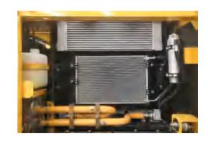
The hydraulic oil radiator, water radiator and inter-cooler are placed horizontally in parallel, which is effective in heatdissipation and easy to clean.
