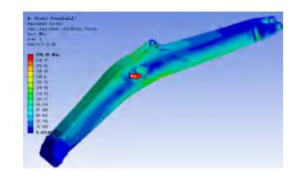
The stress analysis can improve the intensity and stiffness of the boom and arm, which can meet the heavy-duty works, and the machine is more durable and reliable.
