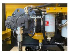
Fuel filters and oil filters are put in proper location, which is much easier for maintenance.
